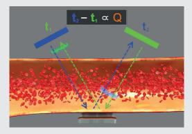
The TTFM principle is based on measuring the difference between upstream and downstream transit time of a wide ultrasound beam. The transit time difference is directly proportional to the blood volume flow. This measurement principle gives an accurate quantification of the real time volume flow that complements the ultrasound imaging.
