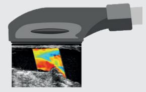
Ultrasound imaging generates images by transmitting ultrasound pulses and receiving echoes from the pulses as they travel through the body. The received echoes are used to create an image of the target area. The color flow mode uses the Doppler principle to detect and visualize blood flow. Pulsed Wave (PW) Doppler uses the same principle to estimate blood flow velocity.
