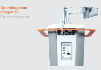
Connect to an external overhead screen using the easily accessible DVI port located on the media panel. The MiraQ<sup>™</sup> Cardiac software has native support for configuring screen size and resolution.
